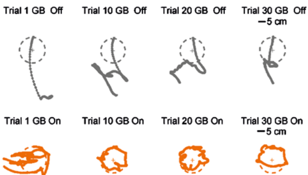
Figure 3: Example data from one stroke patient as she attempted to trace a circle 30 times, without arm weight support (GB) (top) and with arm weight support (bottom), using T-WREX (ArmeoSpring). © 2006 IEEE. Reprinted, with permission, from [14].
