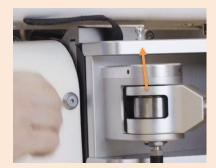
7. Open the clamping lever by pulling the locking pin down and by swinging the lever out until locking pin clicks back into place.
